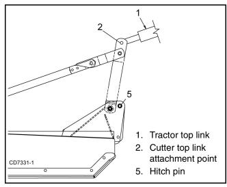
Figure 2. Cutter to Tractor Connection
